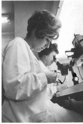
To meet own exacting requirements, F&T East developed and manufactures own electron multiplier. Clean-room assembly is handled by Rita Dunbar at microscope, and Gwen Rafferty. Other beam tube manufacturing operations at the Beverly plant include brazing, welding, vacuum processing.
