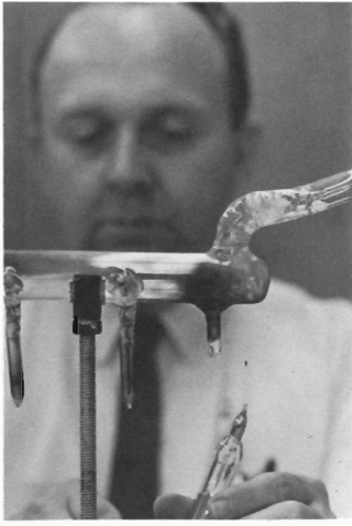
Distilled cesium is removed in flask by Allan Gerrard. Problem is to maintain highly reactive cesium in total vacuum at all steps of manufacture. A small ampule eventually will be inserted inside beam tube. A unique motion within the cesium atom is basis for use as ultra-precise time standard.
